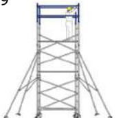
Erect guardrails and horizontal braces. Guardrails should be 0.5m and 1.0m above the platform in all cases.
